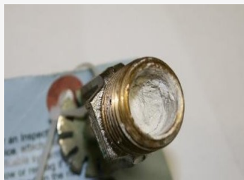
MIC forming bacteria can form "white rust" when in contact with bronze and brass and foul fire sprinkler heads and components
